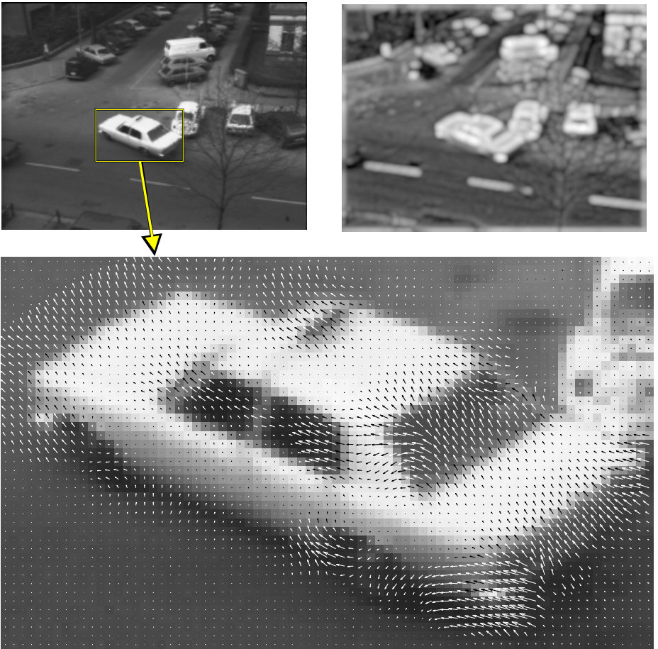
Fig. 6. Experiments on the taxi sequence. Upper left: one frame of the sequence. Upper right: confidences of the estimates in logarithmic scale (white means high confidence). Bottom: estimated flow field for a smaller region of the frame.
