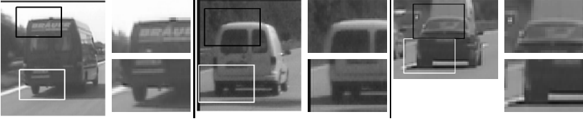
Fig. 1. Variation in the vehicle class of objects is shown. While objects shown here have a drastically different appearance as a whole due to the varying height and type of the vehicle, their components tend to be very homogeneous and are easy to model.
