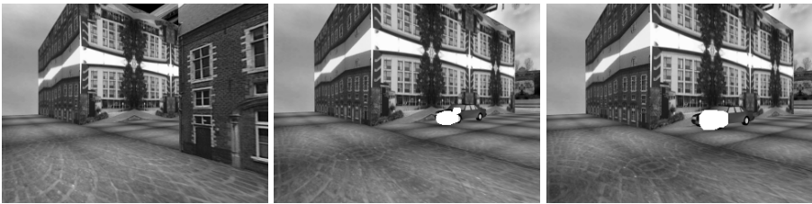
Fig. 8. Some images from the synthetic intersection sequence. The camera is moving on a straight line, while the car in the image is on a collision course. Points where the filter output is above a threshold of 0.35 are marked white.
